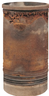
Left undetected, corrosion (as shown on this cylinder liner) can cause costly damage and downtime
